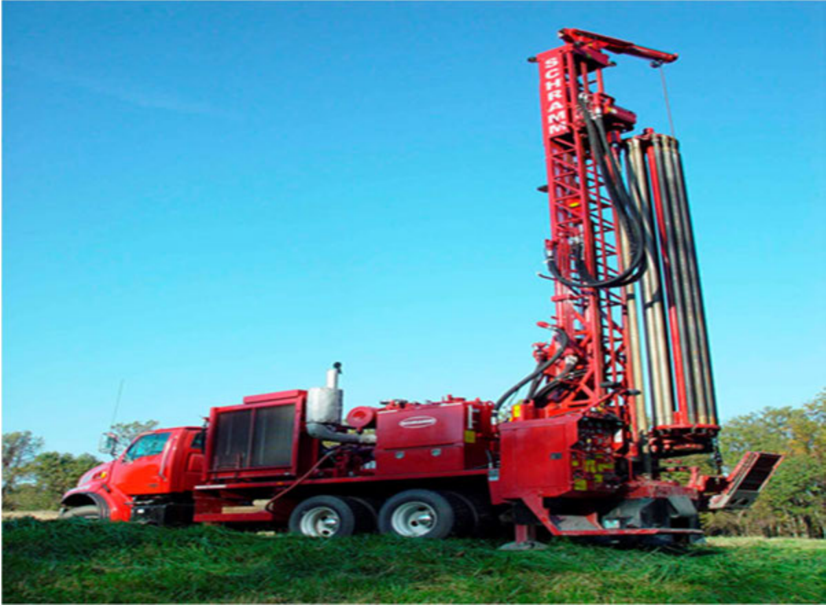
Rotary well drilling rig with raised derrick.
